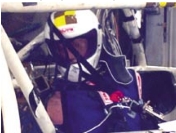
Safety Solutions CSR Window Net with Hans Device. Photo courtesy of Wayne State University.
